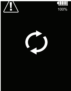
Fig. 35: Clearing symbol (sensor saturated with gas)
