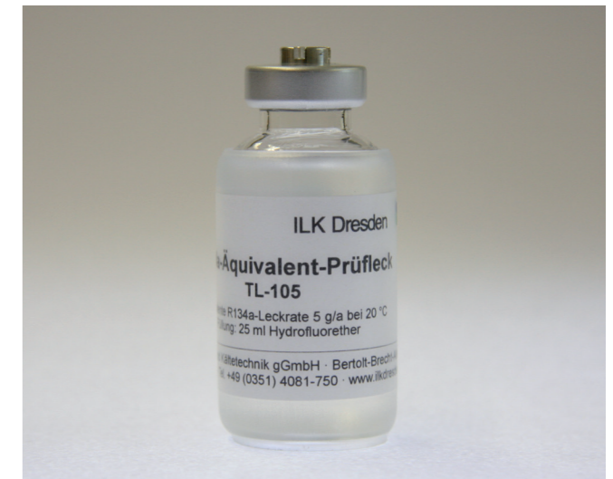
R134a-equivalent reference leak for mobile leak detectors TL-105
